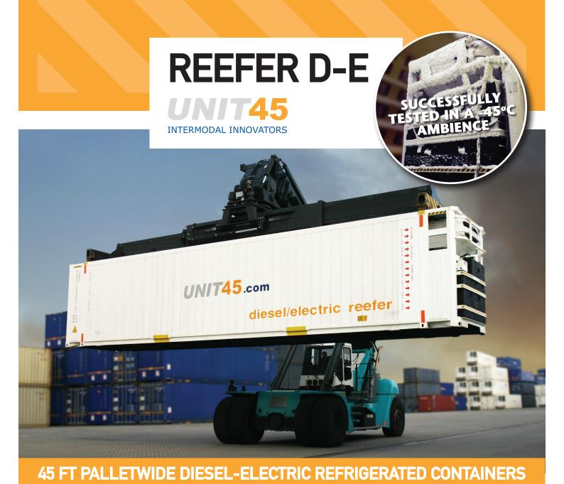
UNIT45 has recently developed a new dieselelectric reefer intended for use in multimodal operations where rail is featured. The cost of moving temperature-controlled cargoes over long distances by road is ever rising but rail is rarely an alternative since very few train operators can provide a reliable power supply
